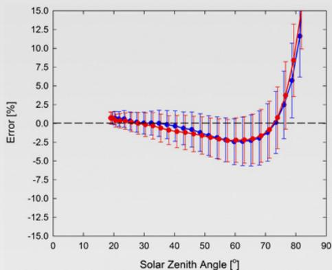
Mean cosine response of twenty-three JSQ original quantum sensors (**error bars represent two standard deviations above and below mean**). Cosine response measurements were made by direct side-by-side comparison to the mean of four reference thermopile pyranometers, with solar zenith angle-dependent factors applied to convert total shortwave radiation to PPFD. Blue points represent the AM response and red points represent the PM response.
