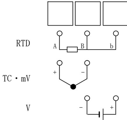
※ In case of mA input, use 250Ω shunt resistor and wire at the area where V input is located.
